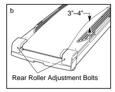
sert the key and run the treadmill for a few minutes. Repeat until the walking belt is properly tightened.
